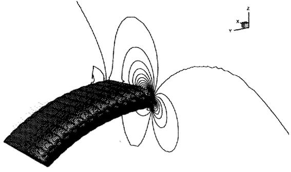
Figure 22. Aerodynamic computation on the deformed structure.
