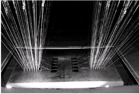
Figure 5. Perforated plate and rigging implementation
