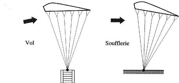
Figure 17. Comparison between flight and wind tunnel configurations
