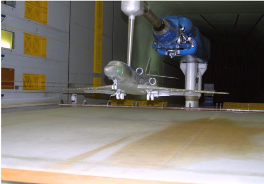
Figure 30. F7X wind tunnel testing with ground effect.
