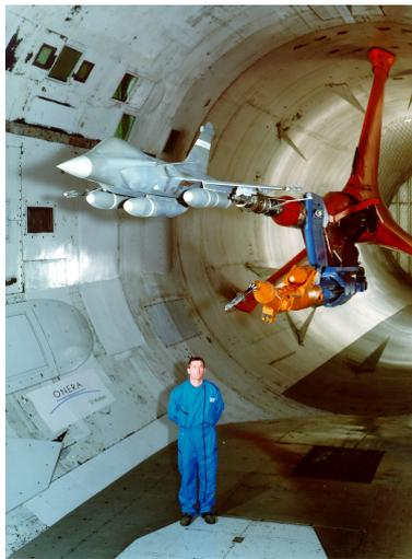
Figure 20. Store release testing at S1 Modane.
